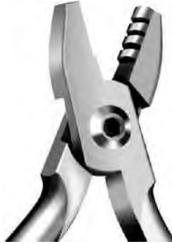
De La Rosa KI- 12-3312 11.5 cm/ 4½" Arch Forming & Contouring Plier With three grooves, for wires .016" (0.41 mm), 0.81" (0.46 mm) and .022" (0.56 mm).
